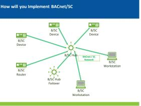
BACnet/SC – Failover B/SC ••• B/SC Device ••• Device B/SC Device B/SC Hut BACnet / SC Net B/SC ••• Workstation B/SC -0-Router B/SC Hub Failover B/SC Workstation
