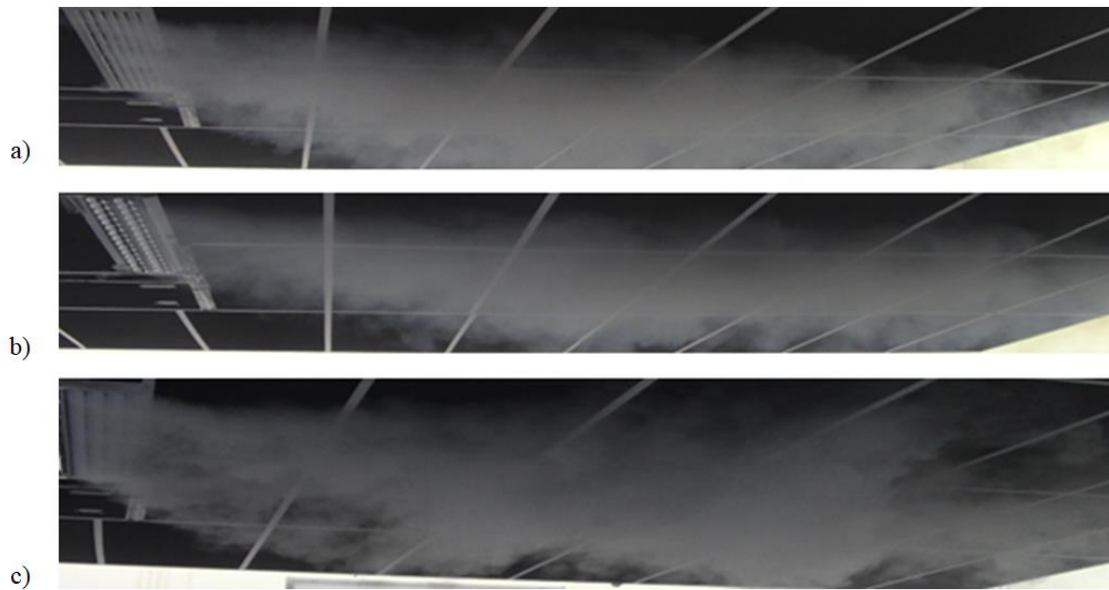
Figure 3 Smoke test of the diffuser, with horizontal air discharge: (a) diffuser no.1, (b) diffuser no.2 and, (c) diffuser no.3.
